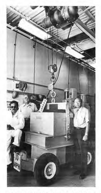
LEAD FILLED TRAILER weighing 18,750 lbs. is saving Sandia time and money in testing hoists in Area III. The trailer replaces large concrete blocks and several pieces of heavy equipment previously used. Idea was conceived by Marv Austin, right. Tom Sanchez, left, designed the trailer and helped Pat Lerma build it from salvaged parts.
